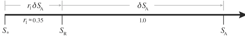
Figure A.4.1. Number line of salinity, illustrating the differences between Preformed Salinity S_* , Reference Salinity S_R , and Absolute Salinity S_A for seawater whose composition differs from that of Standard Seawater.
